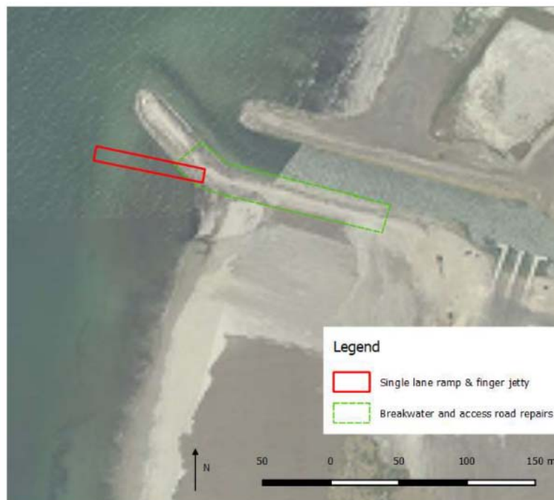
Figure 23: Single lane ramp and finger jetty concept at end of southern breakwater
