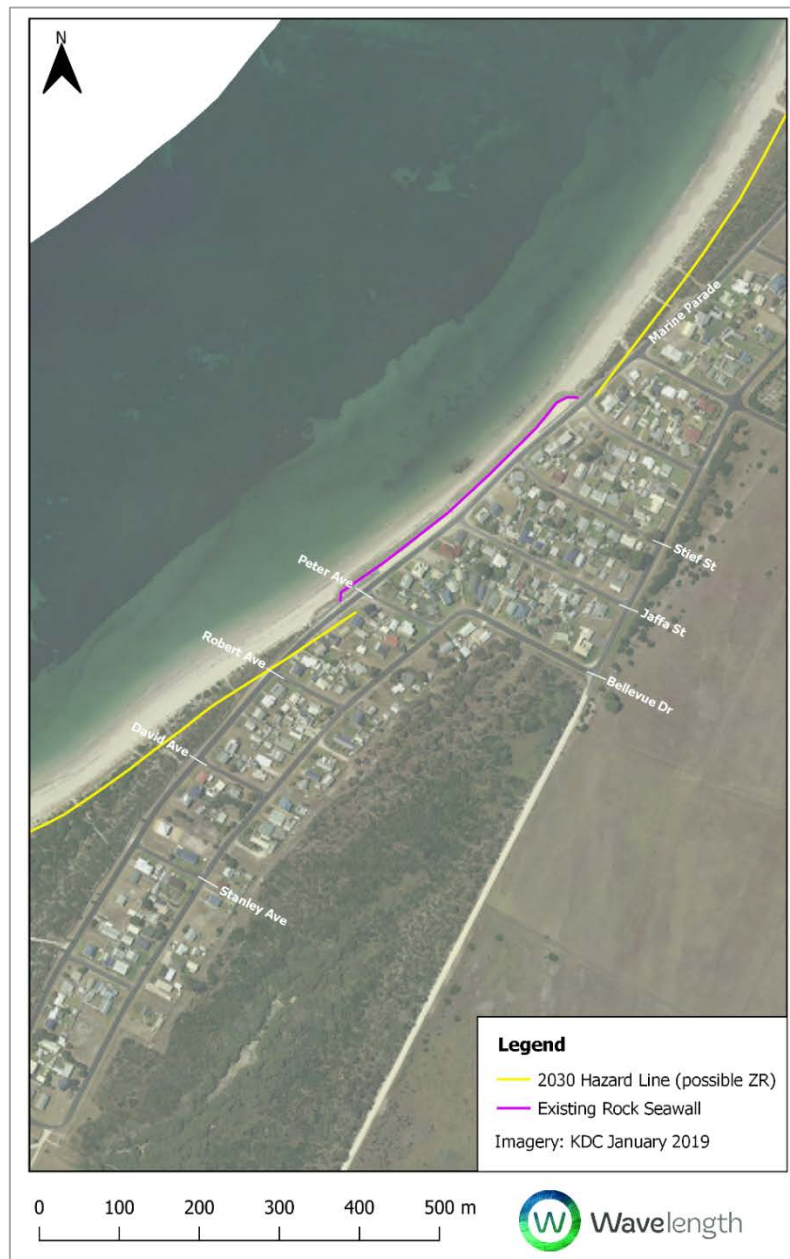
Figure 1 – 2030 Possible Zone of Recession (ZR) Hazard Line
