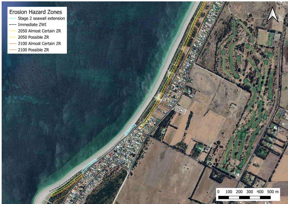
Figure 3-2: 2025 Coastal Erosion Hazard Lines: Wyomi (Section 4)
